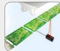
BGS-2S30NT/PT for longer distance. Timer type (0-100msec)
